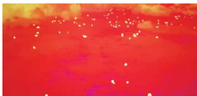
The drone can detect feral herbivores, such as camels, donkeys and kangaroos (pictured). Ambient heat can be seen on the ground area where kangaroos have been lying down (or even standing) for long periods of time. Photo: Autonomous Technology
