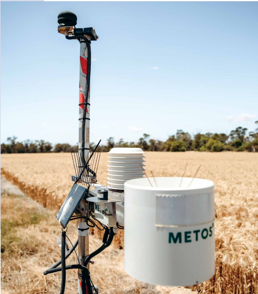
Participating growers were equipped with soil moisture and weather monitoring technology to monitor their focus paddocks. Photo: AGSOCIAL
