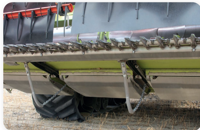
Figure 1: HDPE cable tied to finger tynes. (Glen Riethmuller, DPIRD).
