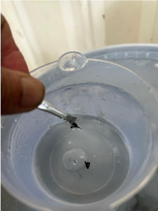
Image 7: a flake of solid SBPM not soluble in water
