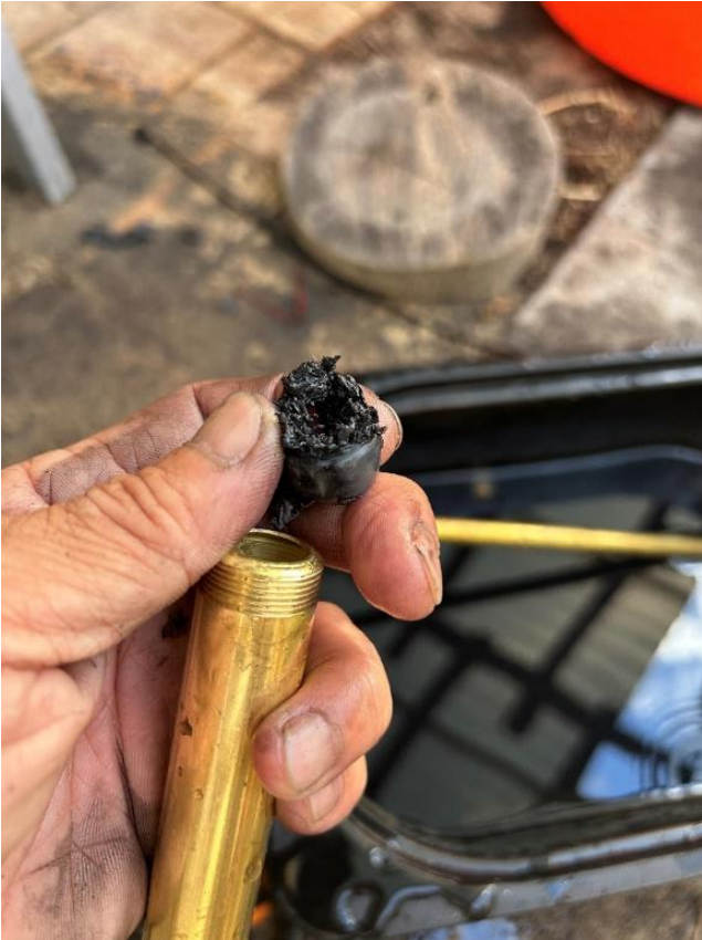
Image 8: Dried SBPM residue formed within a spray nozzle
